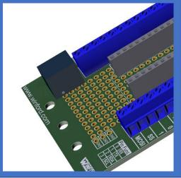
Now, simply plug the Arduino MICRO into the RDBKMIC1 breakout board, and provide power (24V) to the X1 terminal block position. This will provide power to the input of the DC-DC converter, and the DC-DC converter output will provide 9V to VIN on the Arduino MICRO.
