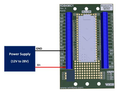
(Note that the power supply must be connected to terminal block position X1, not VIN!)
