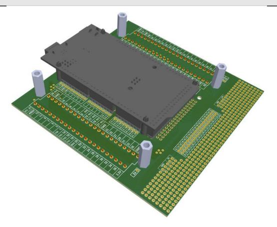
The final assembly (Arduino MEGA2560, RDBKMEG1 Breakout, and Locking PCB Supports) is shown in the figure below.
