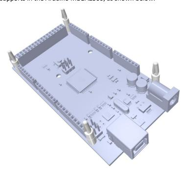
In particular, note that the shorter locking end snaps into the Arduino MEGA2560, and the longer locking end (bayonet style) will interface with the RDBKMEG1 breakout board.
