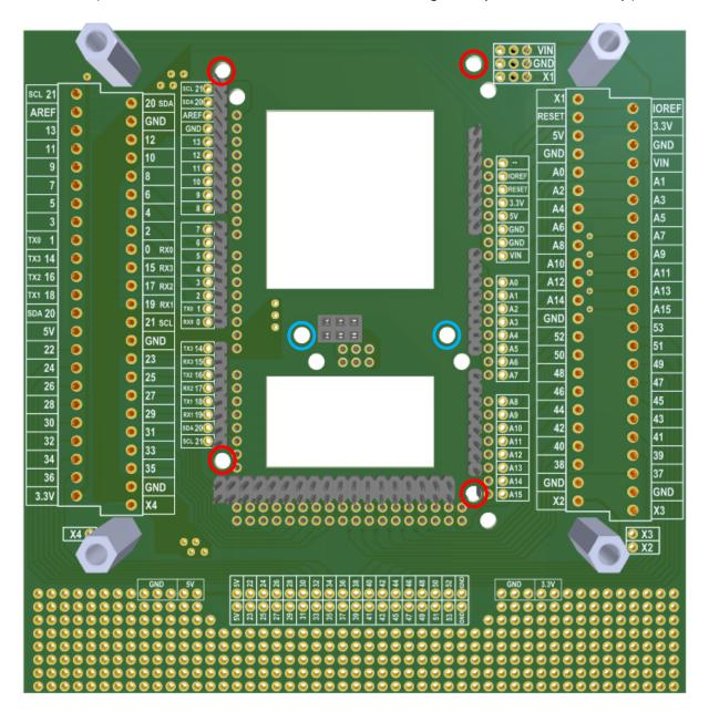
Press the boards together. By design, it will take some force to get the MEGA2560 snapped into place. Work carefully, ensuring that the MEGA2560 board in particular does not get significantly bent.
