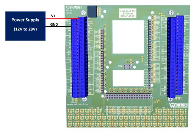
(Note that the power supply must be connected to terminal block position X1, not VIN!)
