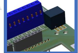
Now, plug the Arduino MEGA2560 into the RDBKMEG1 breakout board, and provide power (24V) to the X1 terminal block position. This will provide power to the input of the DC-DC converter, and the DC-DC converter output will provide 9V to VIN on the Arduino MEGA2560.
