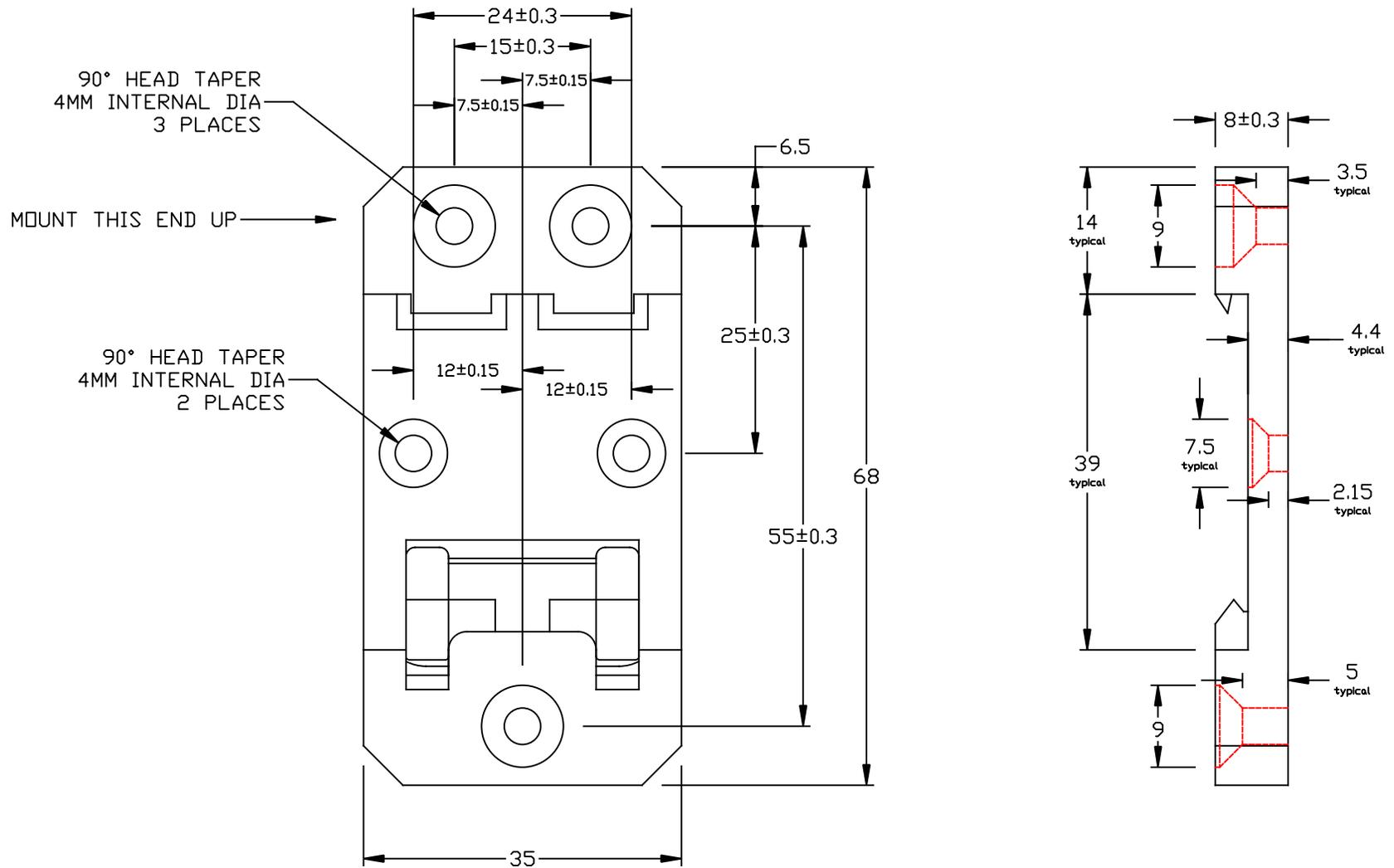
Clip Material: Fiberglass reinforced nylon 66 (PA66+GF30%)
