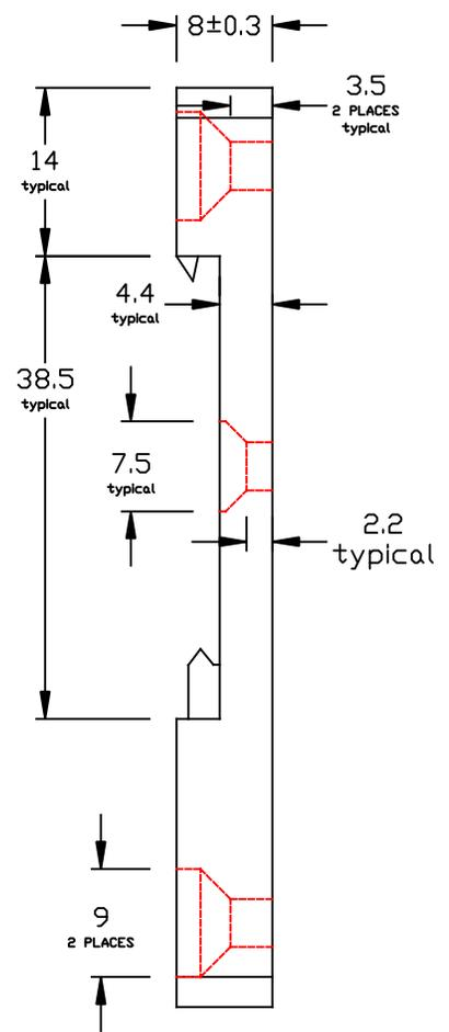
Clip Material: Fiberglass reinforced nylon 66 (PA66+GF30%)
