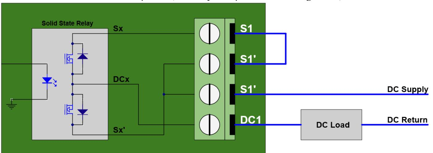
Caution: Note that if DC Supply and DC Return are swapped in the DC configuration, the load will always be powered since current will flow thru the opto-MOSFET body diodes even if the opto-MOSFETs are off.
