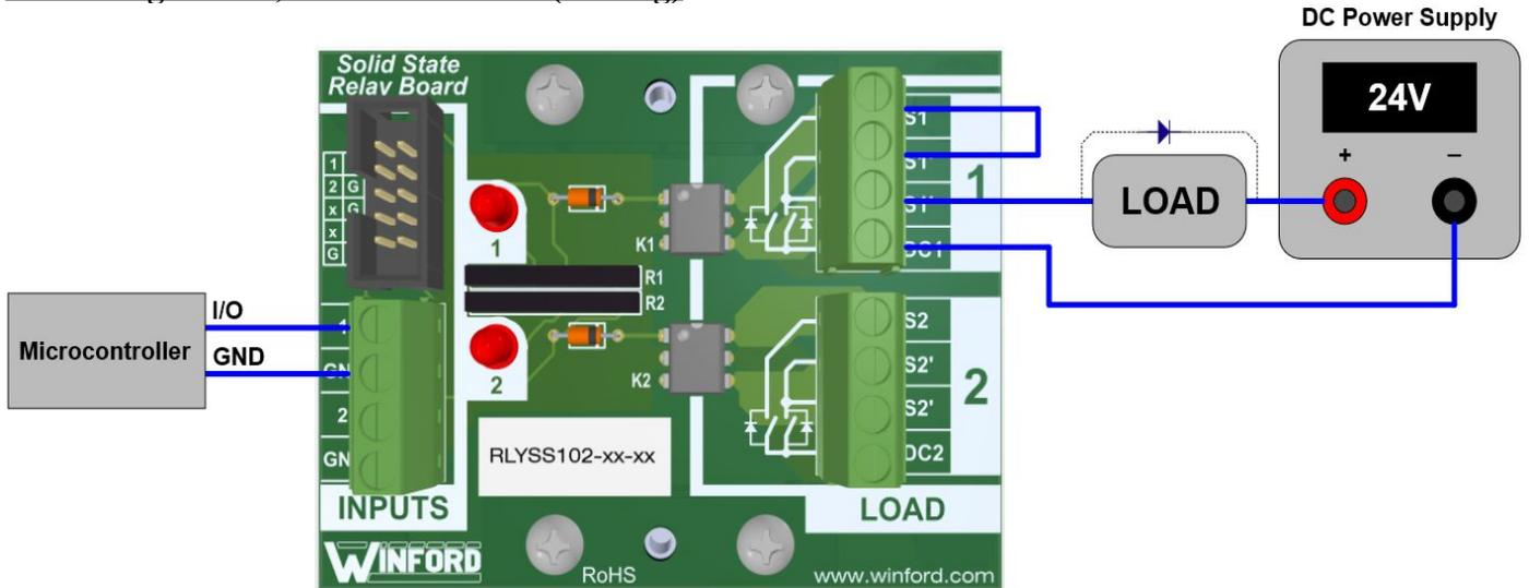
Note that in either of the above cases, the wire connecting S1 and S1' is not needed for low-current loads. It is only needed if warranted by the load current.
