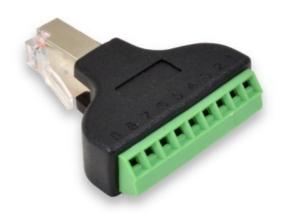
Note that breakout adapters bring all 8 pins plus shield of the RJ45 (8P8C) connector out to screw terminal blocks.
