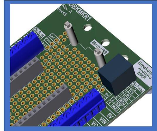
Now, simply plug the Arduino MKR into the RDBKMKR1 breakout board, and provide power (24V) to the X1 terminal block position. This will provide power to the input of the DC-DC converter, and the DC-DC converter output will provide 5V to VIN on the Arduino MKR.
