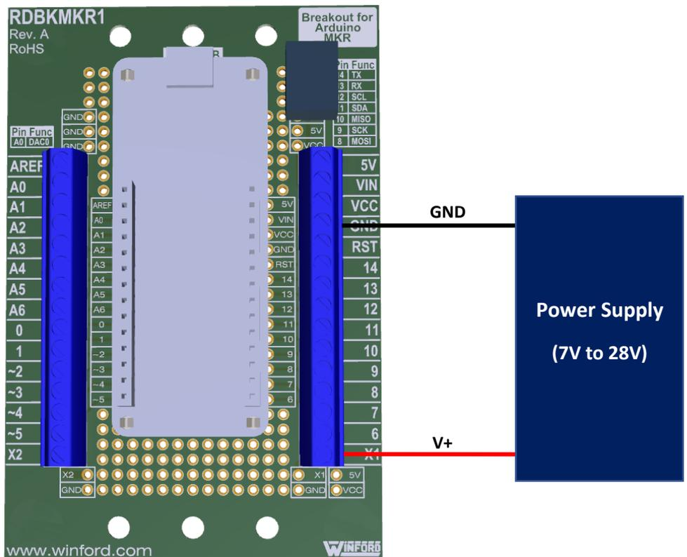
(Note that the power supply must be connected to terminal block position X1, not VIN!)
