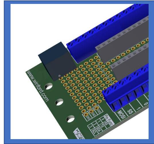
Now, simply plug the Arduino MICRO into the RDBKMIC1 breakout board, and provide power (24V) to the X1 terminal block position. This will provide power to the input of the DC-DC converter, and the DC-DC converter output will provide 9V to VIN on the Arduino MICRO.
