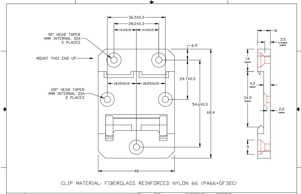
RoHS COMPLIANT: YES DESCRIPTION: DATE: 06-30-2016 6/30/16 Added hole-hole distance tolerances. DIN Rail Mounting Clip, 48mm Width 1/26/16 Added hole depth details; corrected 24.6 dimension to 24.7. Winford Engineering, LLC 4561 Garfield Road No change to physical parts. PART NUMBER(S): PART REVISION: Auburn, MI 48611 DINM15-RC Date 989-671-9721 www.winford.com
