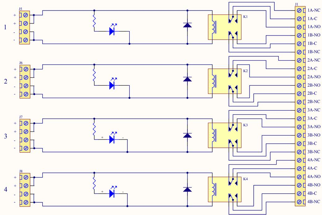
NOTE: This schematic accurately represents the circuit, but some individual components are combined into a single package on the product PCB.
