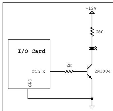
**Figure 1: Basic transistor switch**
