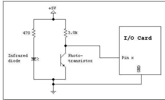
**Figure 4: Open-collector circuit**
